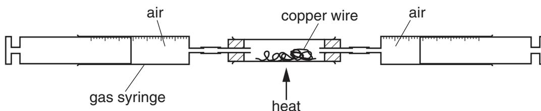
Air is passed backwards and forwards over the heated copper using the syringes. The copper reacts with oxygen in the air.
